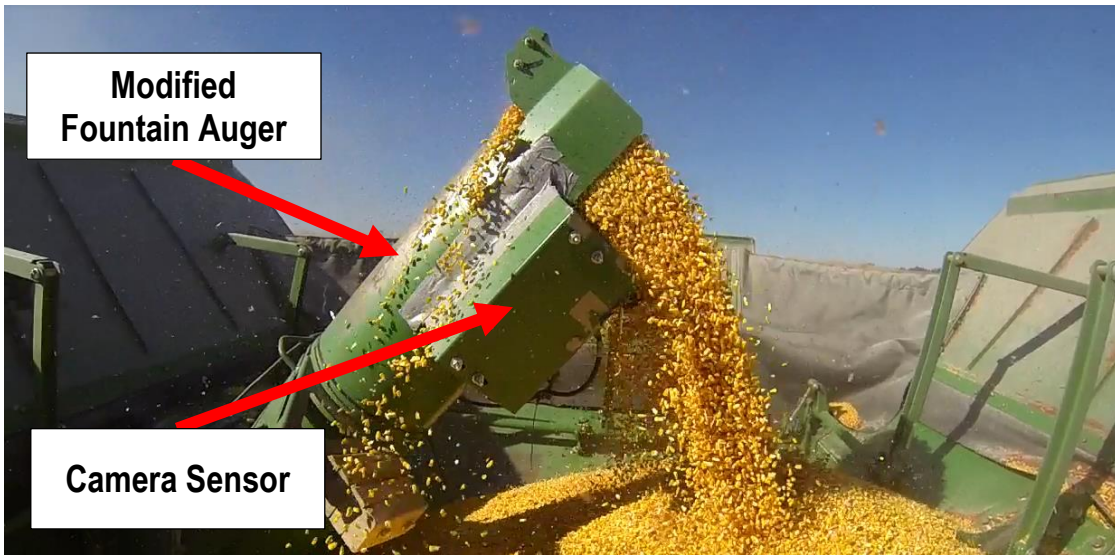
Figure 5.10: Fountain auger modifications of baffles, sump, and tapered auger to deliver grain effectively to sensor
