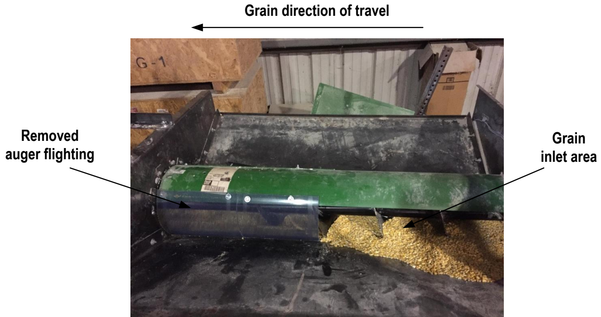
Figure 5.2 : Auger test stand for determination of cavity power requirement
