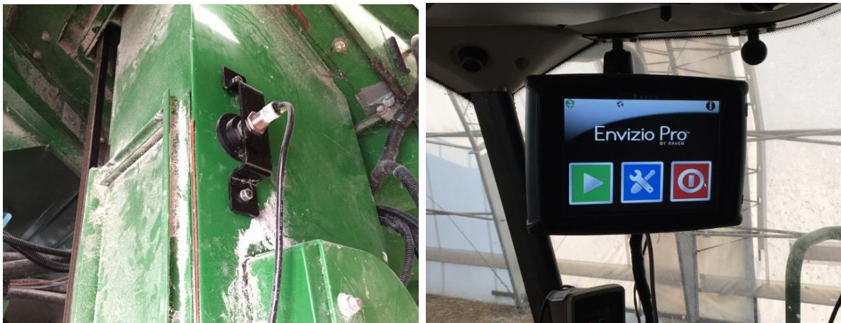
Figure 4.2: SmartYield Pro yield monitor beam-based volumetric flow sensor and display, respectively.
