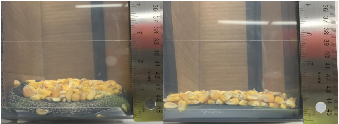
Figure 4.10: Grain pile loading on paddle ID no. 1 and 3 for 5 \text{ kg s}^{-1} mass flow rate, respectively
