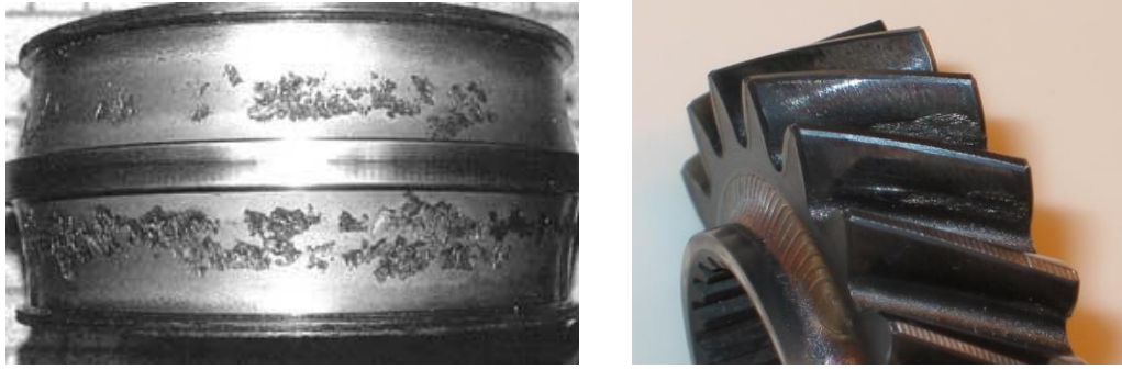
Figure 1.5: Representative images of macropitting phenomena observed in gears (left) [46] and bearings (right) [47]
