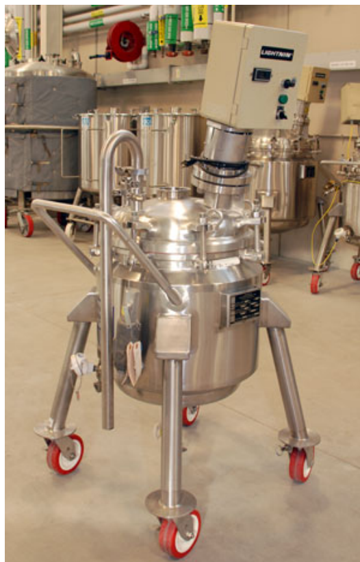
Figure 4.2 Photograph of Feldmeier 70-liter jacketed tank
