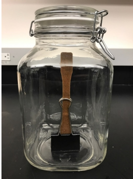
Figure 4.3 Photograph of odor test sample of 3 Liter jar containing molded specimen
