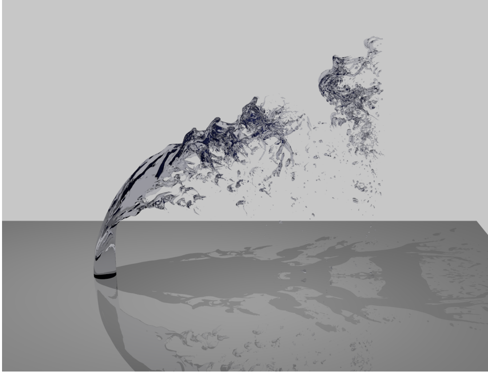
Figure 1.1 Example of the breakup process for a liquid jet in crossflow.
