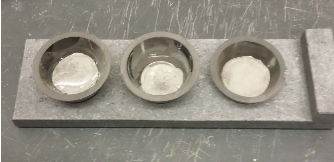
Figure 5 – Graphite boat and glassy carbon crucibles used for nitriding glasses containing nitrided lithium phosphate glass.
