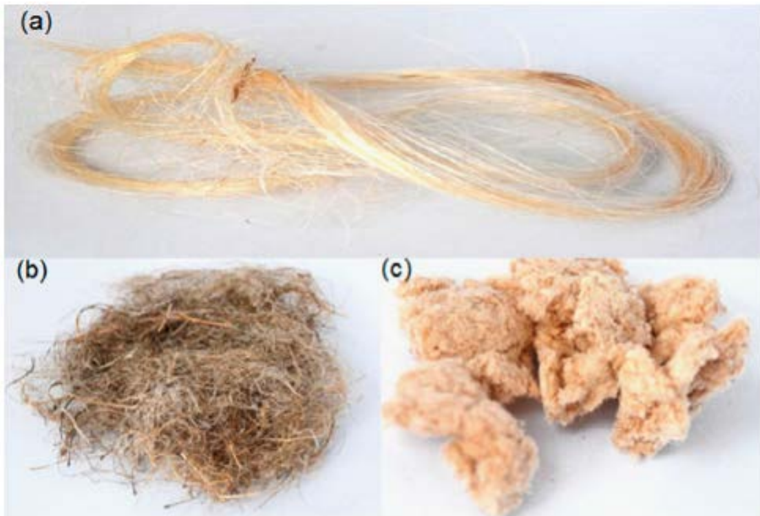
Figure 2.19 a) Strand Fibers , b) Staple Fibers , c) Pulp Fibers (Ardanuy et al. 2015)
