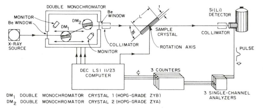
The positions of the crystal and detector on the diffractometer are also computer controlled. The resolution for the "theta" and "two theta" angles as well as for the rotations controlling the position of the analyzer is 8000 steps/degree. The resolution of the two rotations in the Eulerian cradle is 400 steps/degree. In addition, a helium, closed cycle refrigerator having a temperature range of 6.7 to 400 K can be mounted on the diffractometer.
