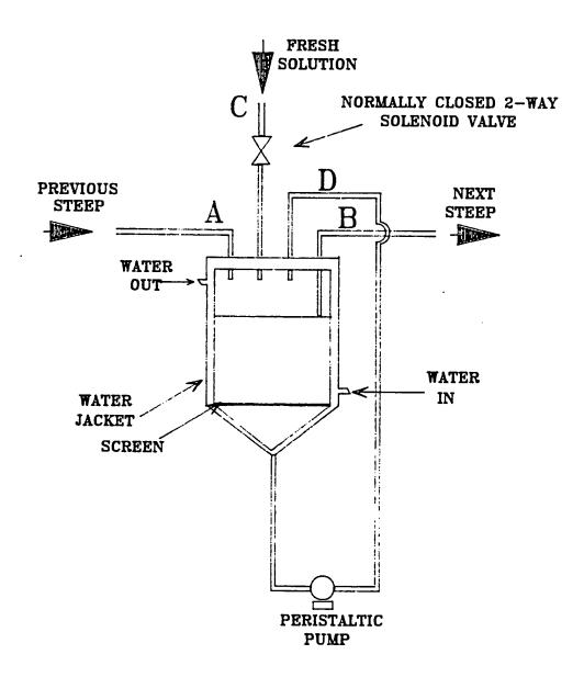
circulation rate to each vessel was equal, thus keeping the same temperature among different vessels. The pumping rate was adjusted by using a voltage controller (Cole-Parmer Inc. model 2603) in order to keep temperature of the steeping at  $50^{\circ}$ C and not over-pressure the tube connections.
