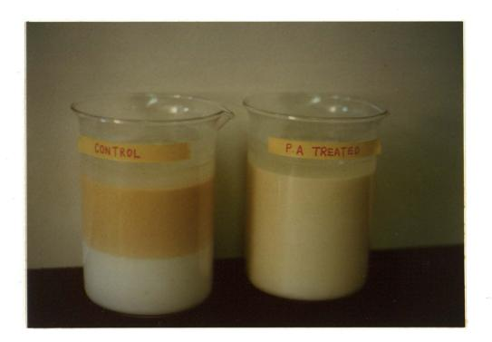
Figure 7. Sedimentation separation of mill-starch from air-dried corn (Control) and corn treated with pure propionic acid (P.A. Treated) (Sample allowed to settle for 10 min)
