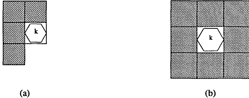
Figure 39. Neighborhood systems (a) N_k \equiv \text{adj}_{\leftarrow} A_k for fourth-order POMM, and (b) \delta_k for second order MRF, represented by the shaded regions.
