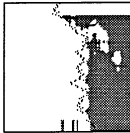
(e) Initial segmented image I by using local joint probability with neighborhood size 32x32.
