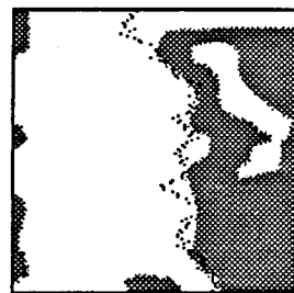
(b) Final segmented image after 257 iterations on image in Fig. 40(c), M_k = 8 \times 8 , update segmented image after 1 scan through whole image. Final temperature 0.18, clique potential, d= 2.5 .
