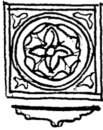
Figure 62. The original metal plate ceiling tile.
