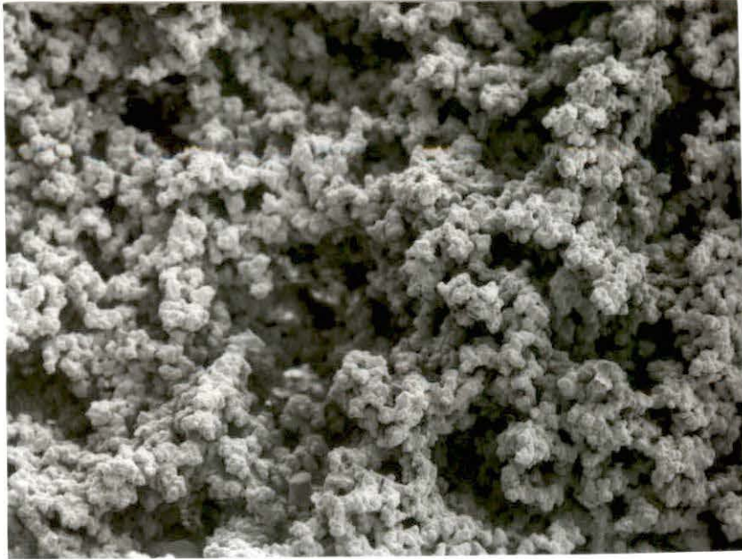
Figure 9. P-HEMA. Sample SIP1 with 10% HEMA - 90% water and initiator (689 kPa (100 psi)), 5 keV, 350X
