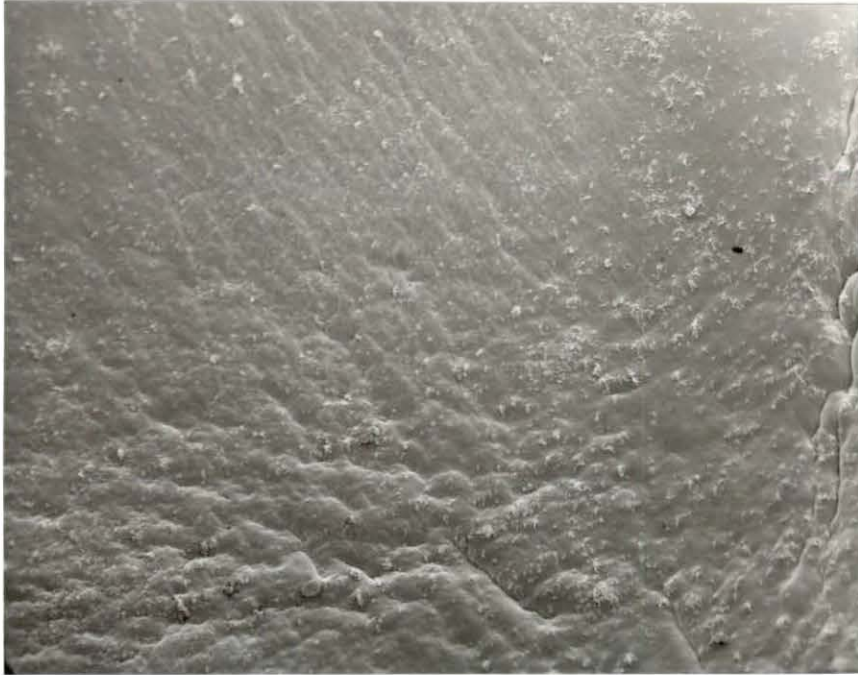
Figure 13. P-HEMA. Sample SIP6 with 60% HEMA - 40% water and initiator (689 kPa (100 psi)), 5 keV, 350X
