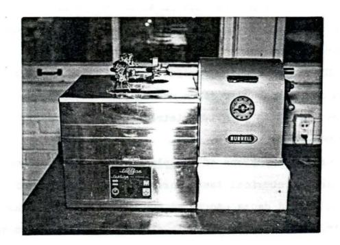
Figure 1. Wrist action shaker and 37°C. water bath employed to grow <u>Mycoplasma</u> <u>hyorhinis</u>
