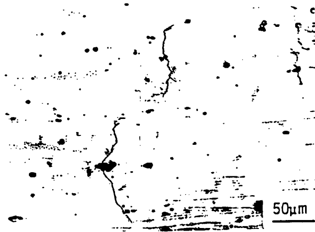
Figure 3.3. Example of fatigue cracks associated with inclusions [50].
