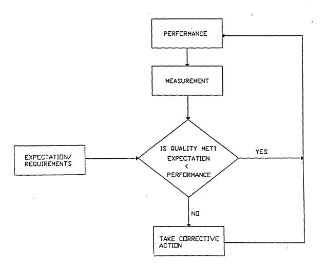
Figure 5. Diagram of the quality control cycle
