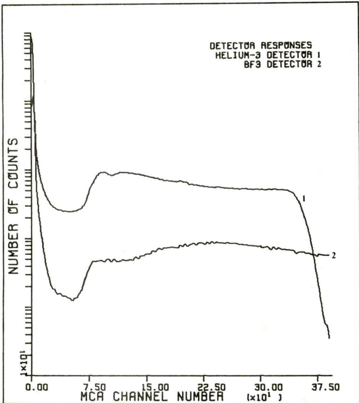
Figure 4.7. Response of  $^3\text{He}$  and  $\text{BF}_3$  detectors to thermal neutrons and gammas
