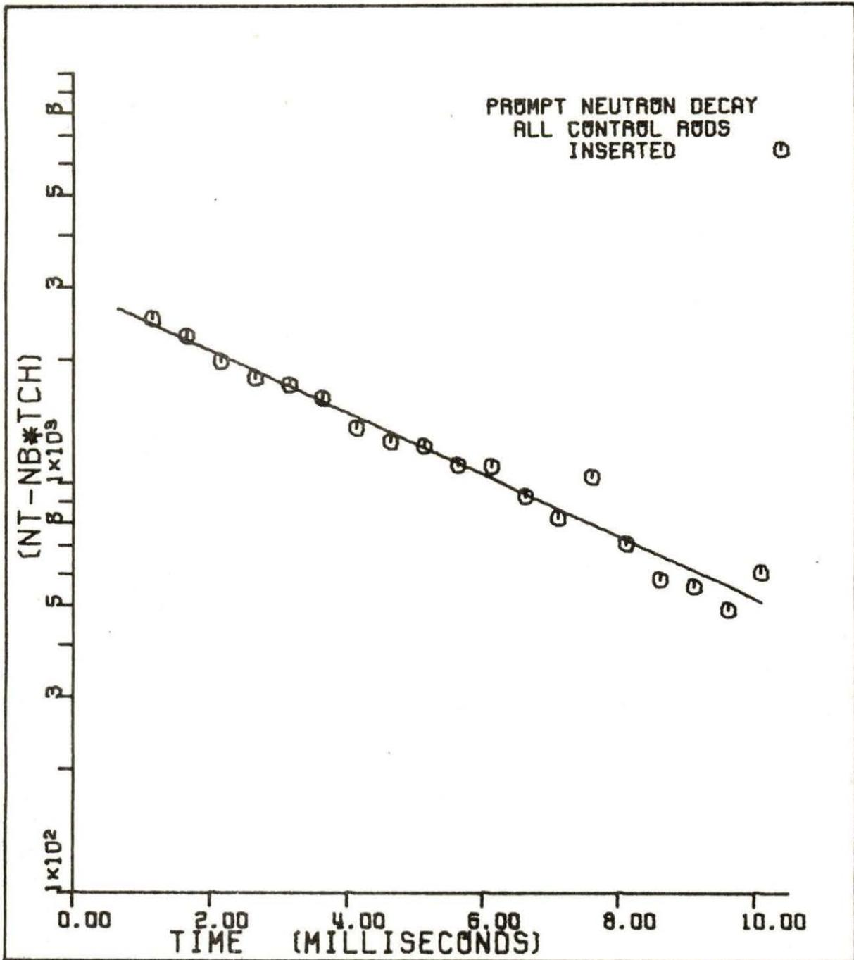
Figure 4.11. Decay of prompt neutrons with all control rods inserted
