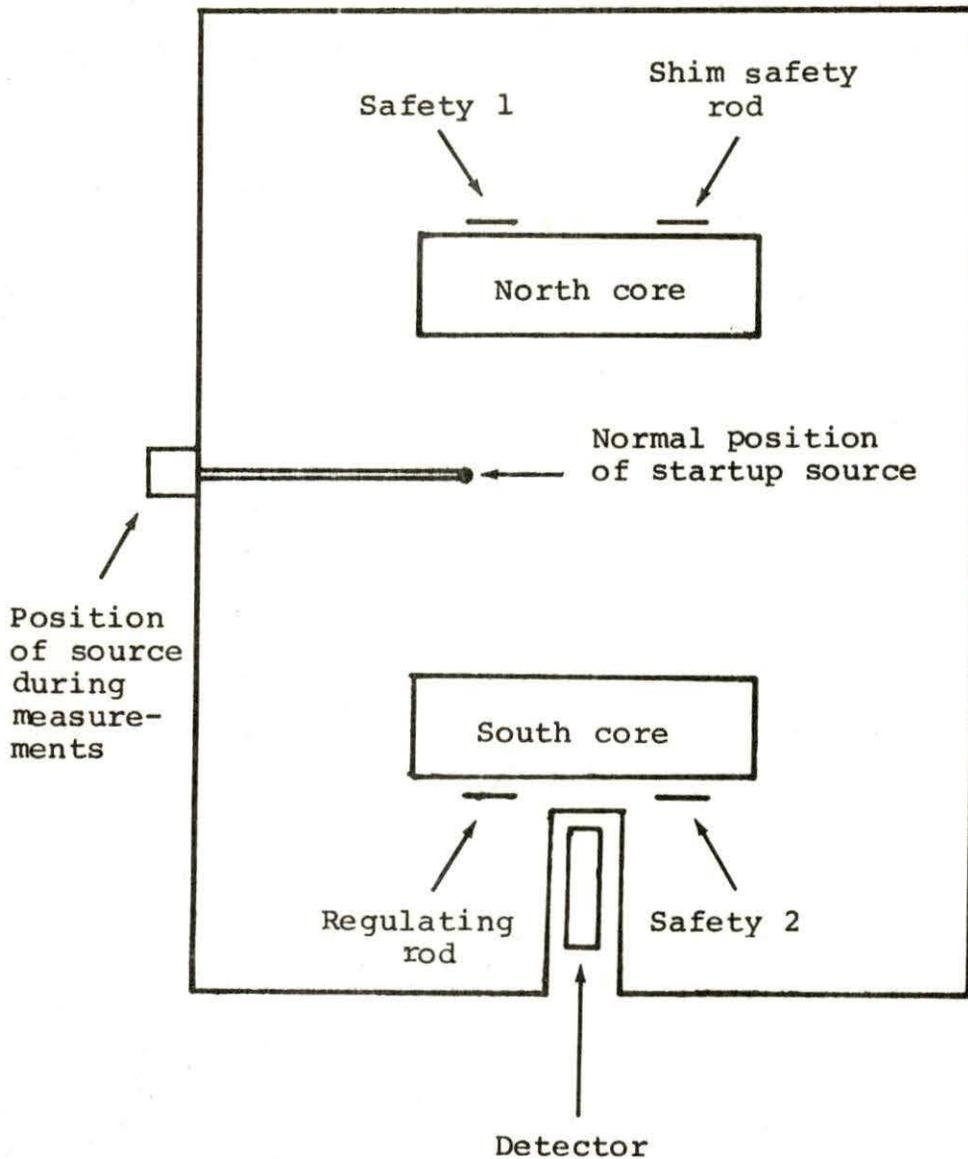
Figure 4.6. Geometrical arrangement of the UTR-10 coupled core reactor
