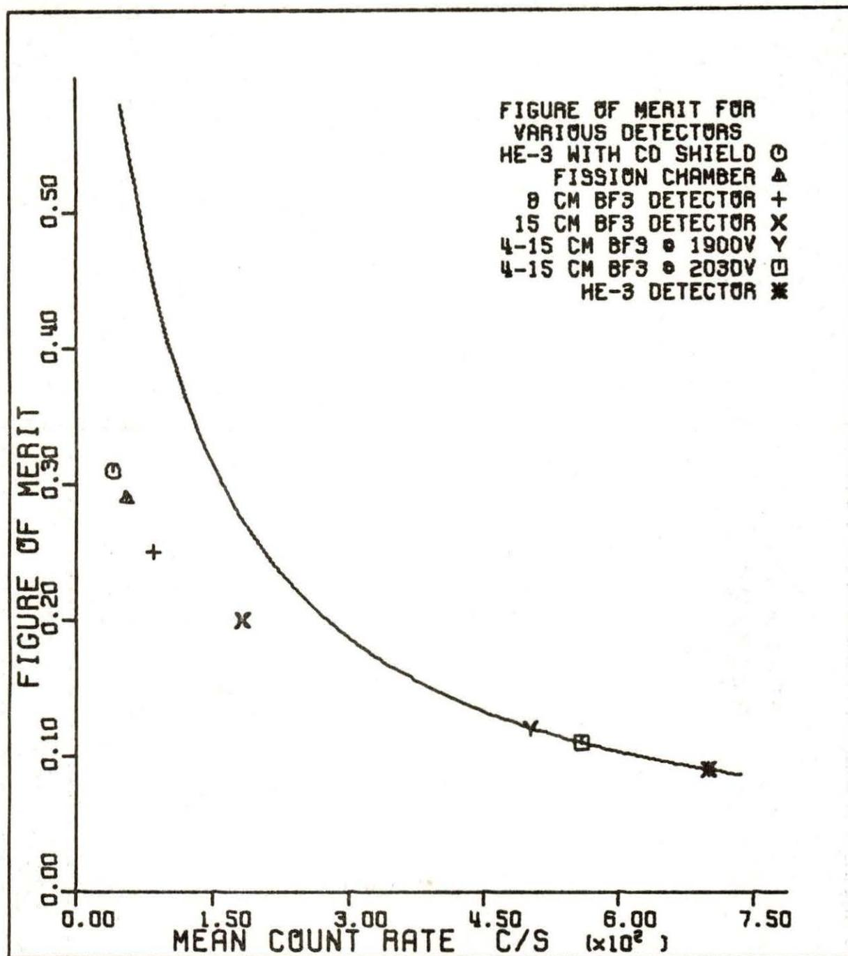
Figure 4.8. Figure of merit for various detector arrangements
