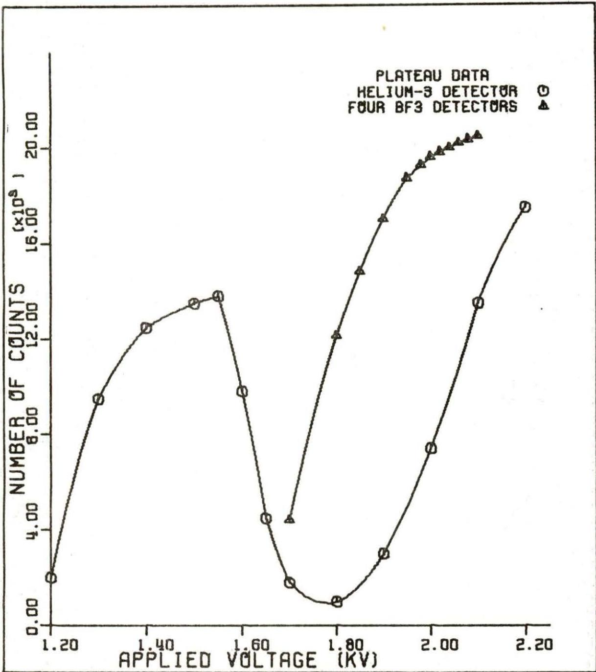
Figure 4.10. Effect of high voltage on count rate for <sup>3</sup>He and BF<sub>3</sub> detectors
