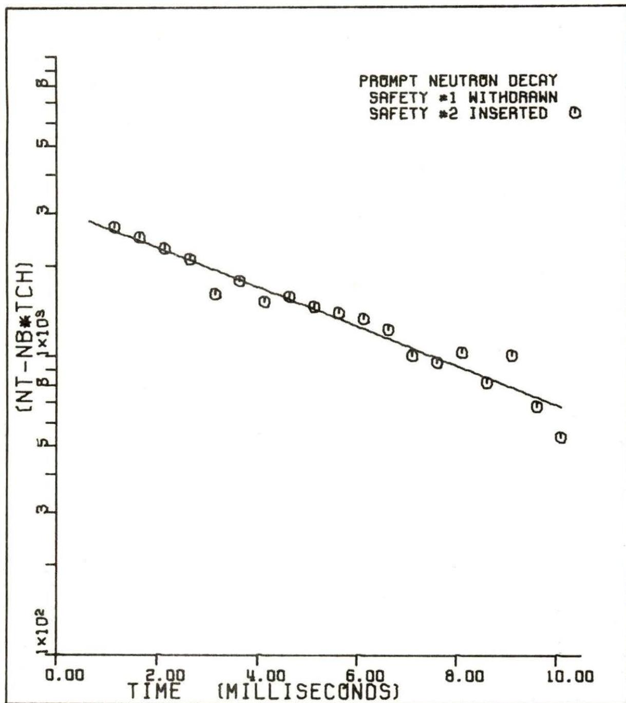
Figure 9.2. Prompt neutron decay with safety 1 fully withdrawn and safety 2 fully inserted
