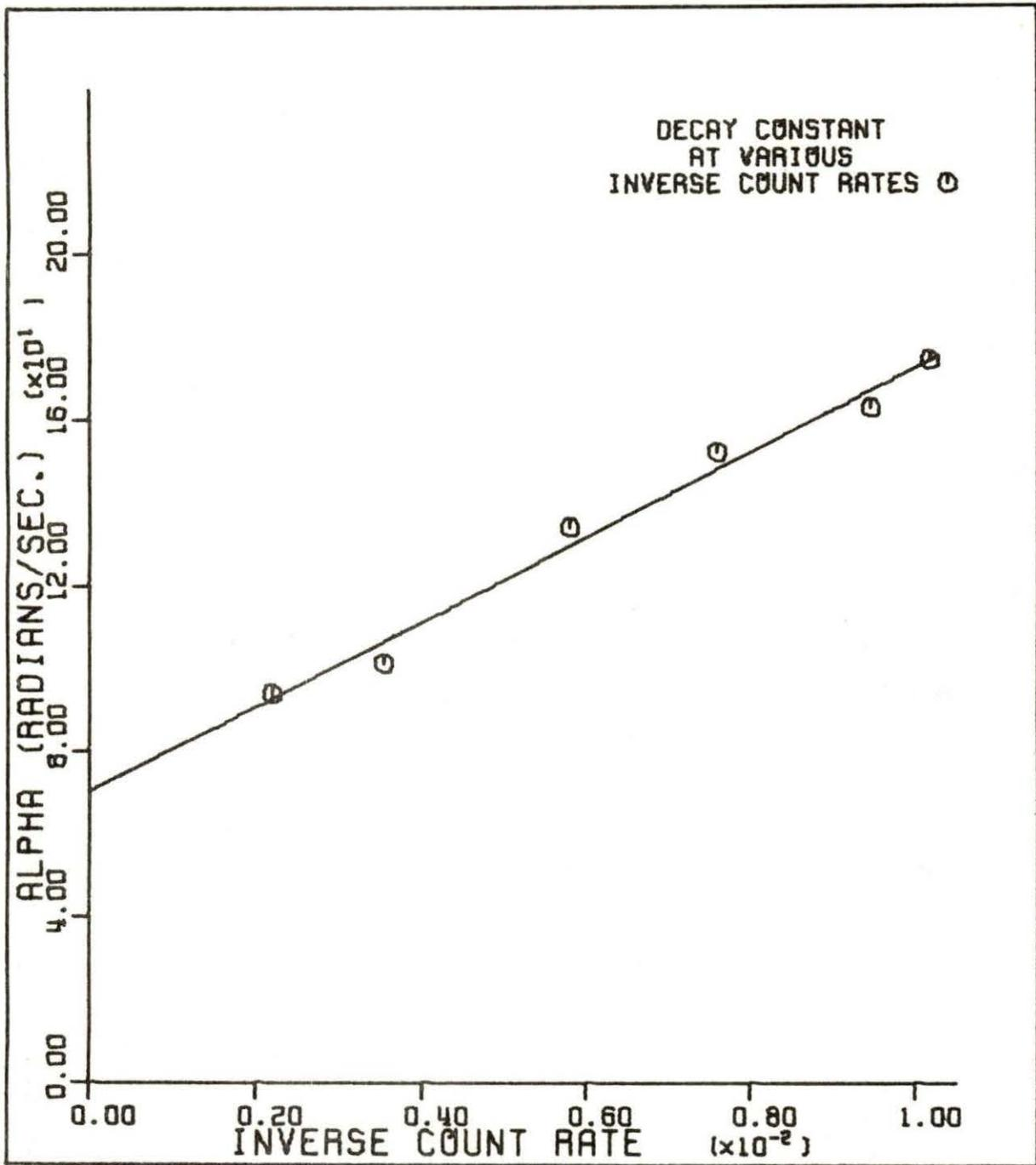
Figure 4.12. Prompt neutron decay constant for various reactor configurations
