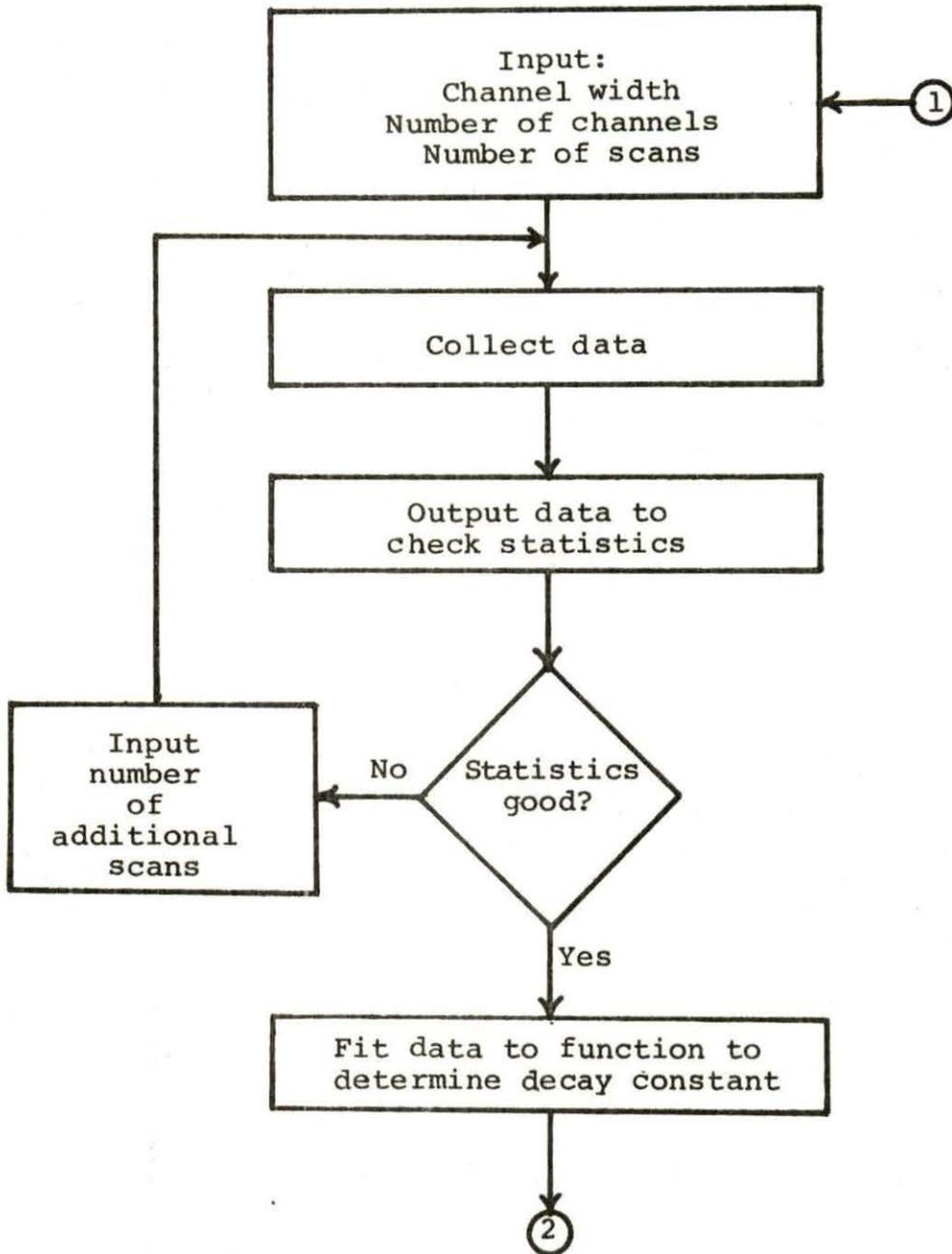
Figure 3.1. Consolidated acquisition-analysis program based on the Rossi Alpha Method
