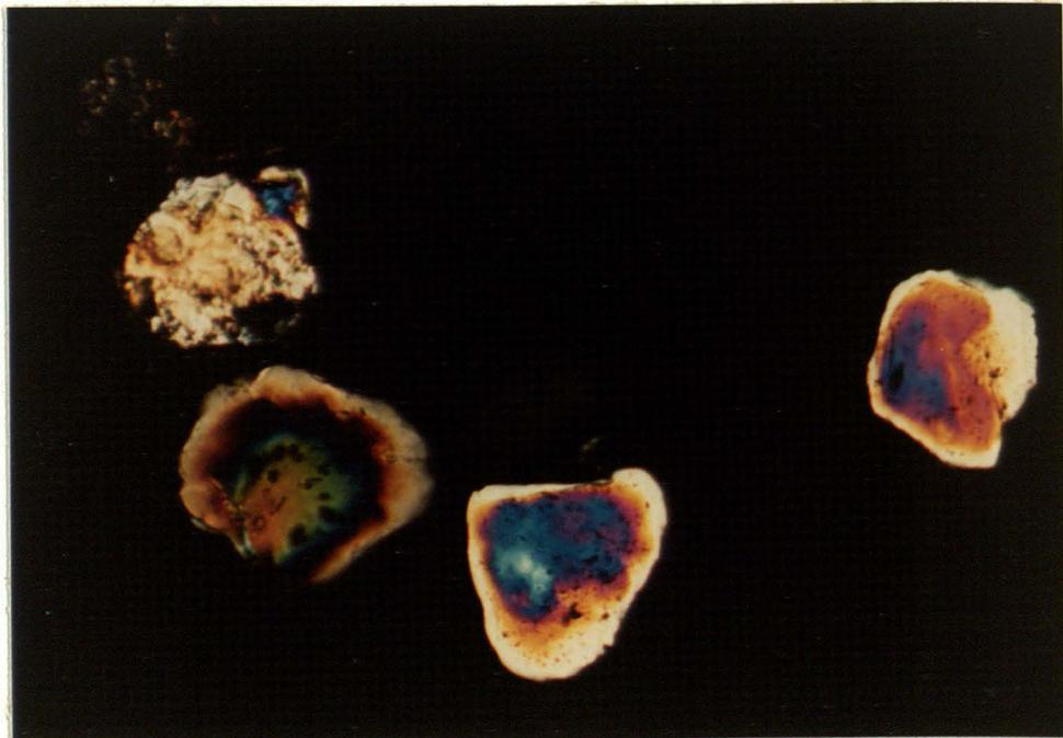
Figure 20d. Quartz crystals with inclusions
