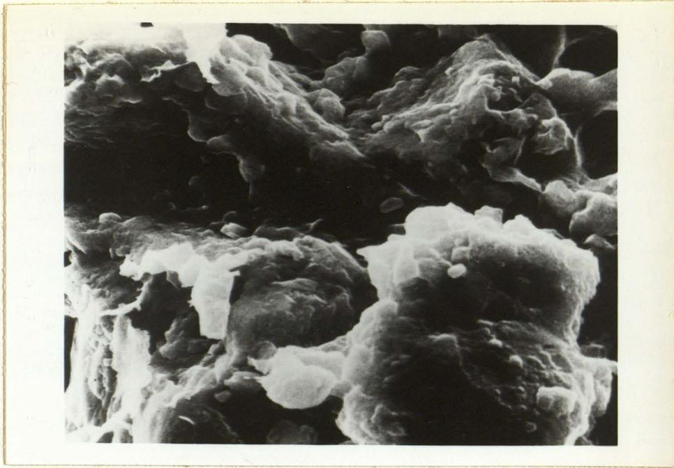
Figure 20c. SEM photo showing quartz overgrowth
