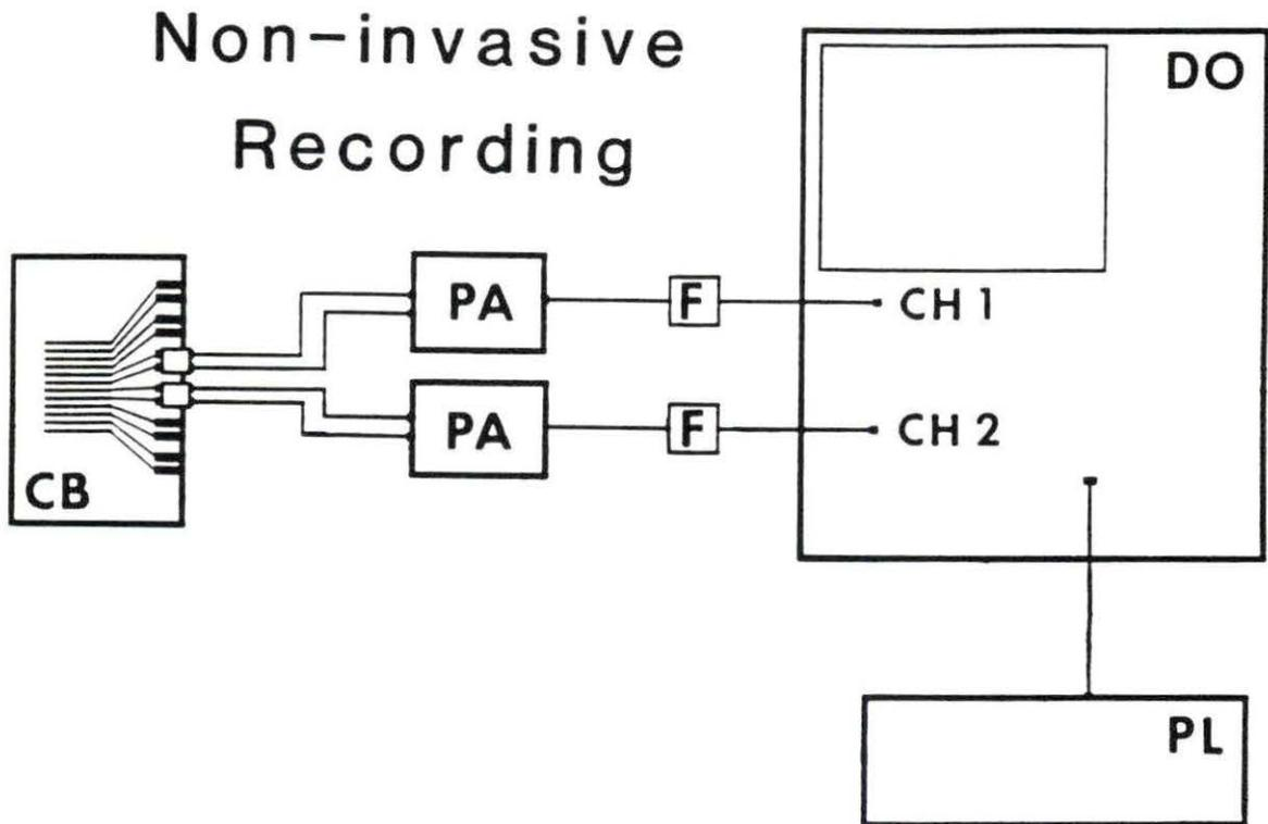
Figure 1. Recording apparatus. CB: Circuit Board, PA: Instrumentation Amplifiers, F: Filters, DO: Digital Oscilloscope, PL: Plotter.
