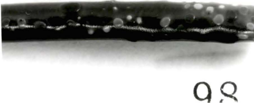
FIGURE 11. Magnified view of the sample prepared using the 80% NVP/20% methanol formulation (200 Krad dose) of Method C
