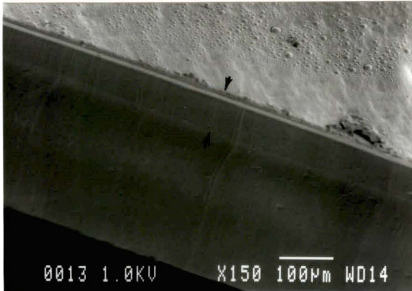
FIGURE 3. Scanning electron micrograph from edge of 60% NVP/40% methanol sample prepared by Method A(ethanol/water rinse) and stained in 10% basic fuchsin in 100% methanol. Arrows denote boundaries NVP graft
