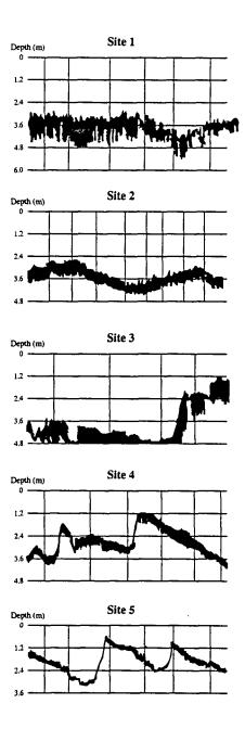
Figure 9. Longitudinal depth soundings made in the main channel of the Missouri River downstream to upstream at all five study sites during the nonnavigation season. Vertical lines show approximately when the boat passed a wing dike.
