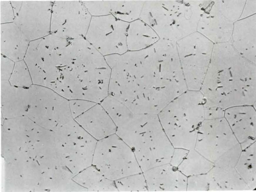
Metallograph 9: \text{La}_{2.7}\text{Sm}_{0.3}\text{S}_4 top of ingot horizontal slice 500X.
