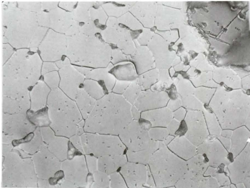
Metallograph 16: \text{La}_{2.3}\text{Sm}_{0.7}\text{S}_4 bottom of ingot vertical slice 500X.
