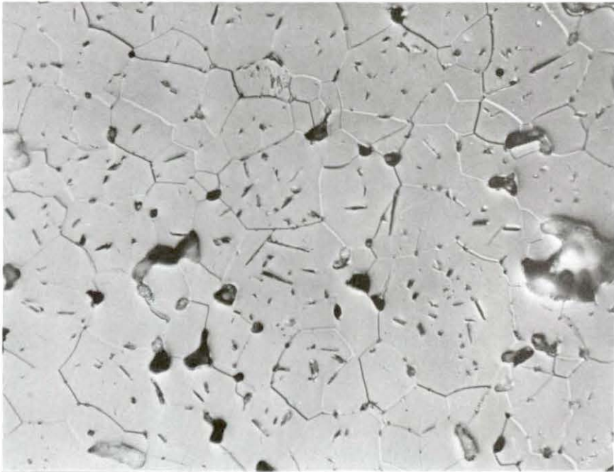
Metallograph 24: \text{La}_{2.3}\text{Yb}_{0.7}\text{S}_4 bottom of ingot vertical slice 500X.
