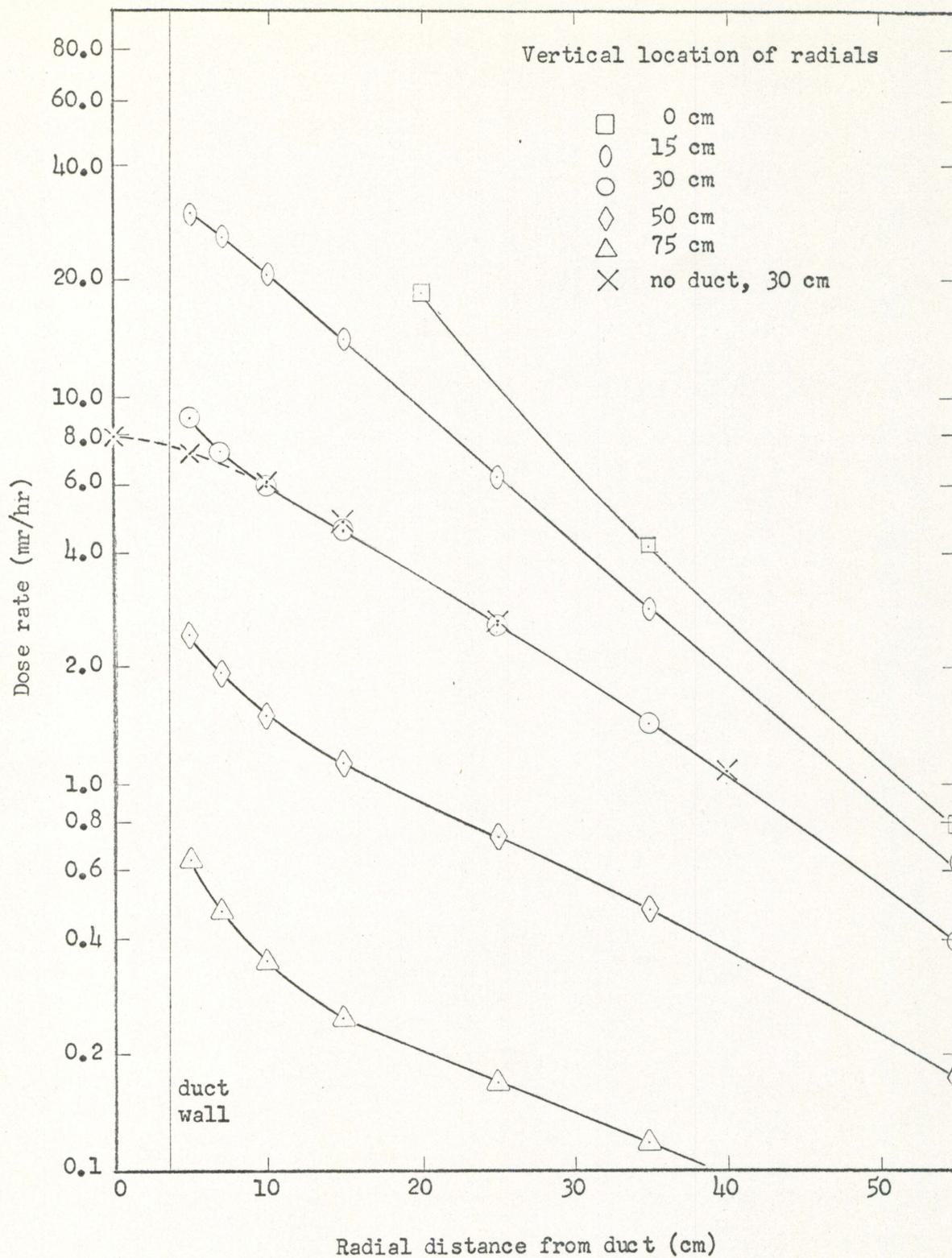
Figure 1. Loss rate as a function of vertical distance from the source
