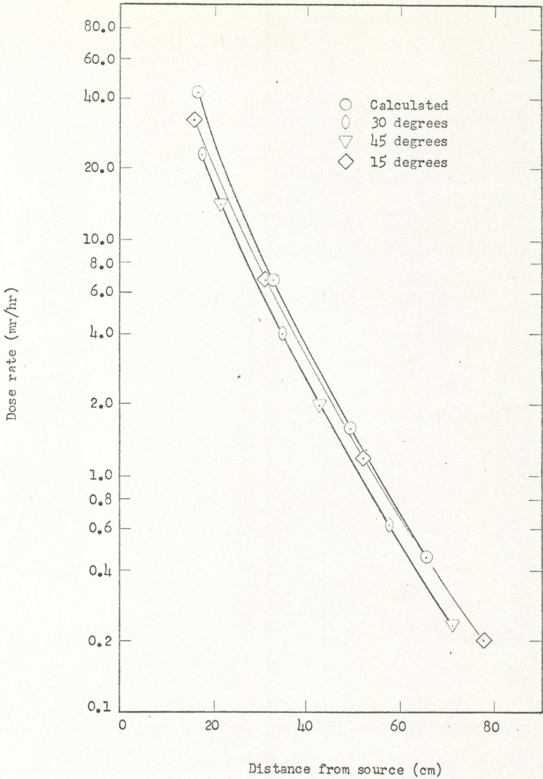
Figure 6. Experimental and calculated dose rates without the dust
