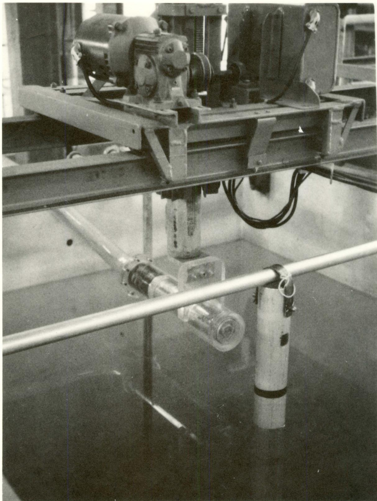
diameter by 1 in. long. A single channel, Nuclear Chicago radiation analyser, model 1810, was used for measuring the energy spectrum. Counting was accomplished with a Nuclear Chicago ultrascaler model 192A-P. The resolving time of the first electronic decade of this scaler was 1 microsec. The maximum count rate was limited by the mechanical register to 170,000 cps.
