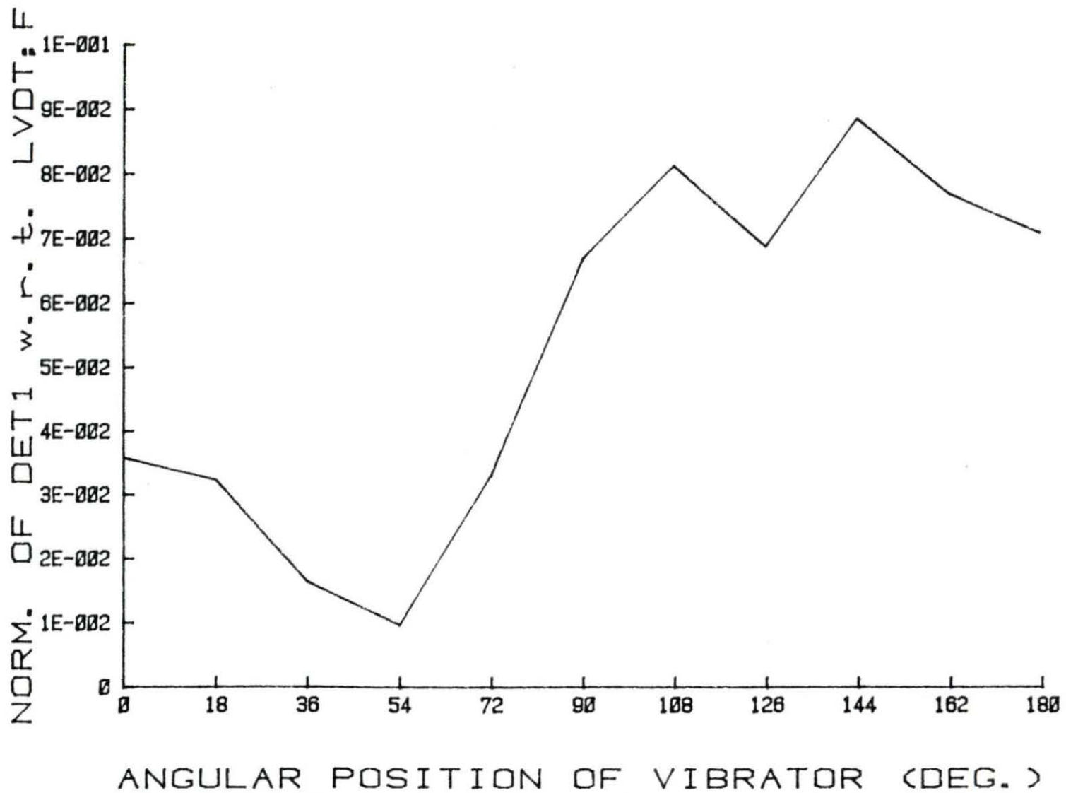
FIGURE 32. Normalization of DET1 to LVDT at 1.52 Hz vs angular position of the vibrator (flooded case)
