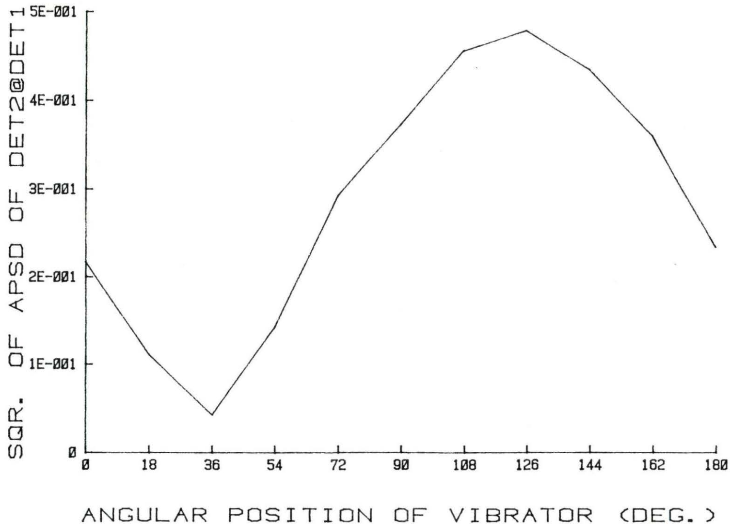
FIGURE 29. Magnitude of DET2 (@DET1) at 1.52 Hz vs angular position of the vibrator
