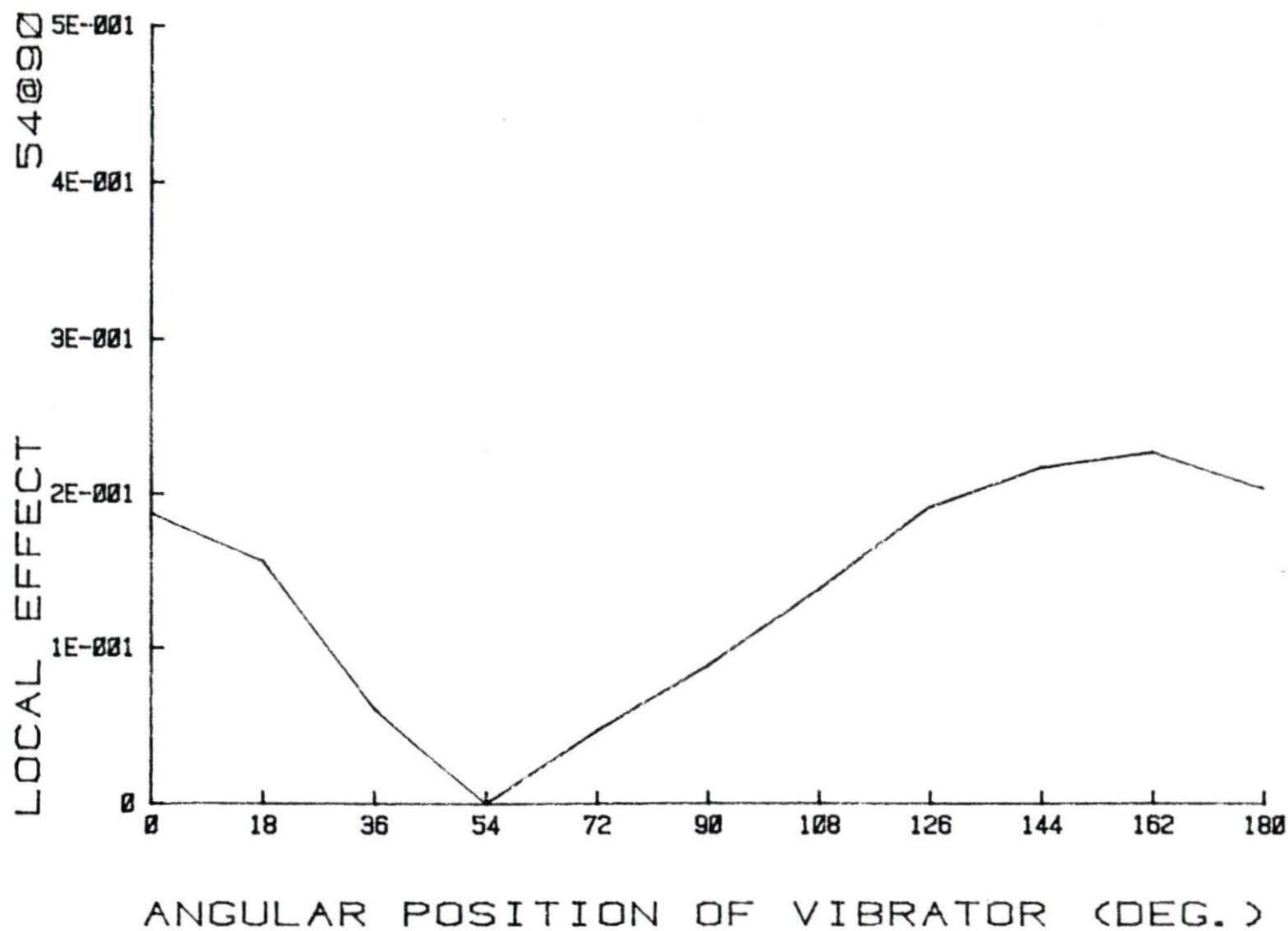
FIGURE 47. Local effect at 1.52 Hz vs angular position of the vibrator
