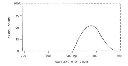
Figure 6. Transmission spectrophotogram of the secondary filter (Jena type OG-1) used in the Leitz Ortholux research microscope adapted for fluorescence microscopy.
