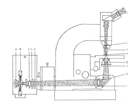
condenser, dry type,<sup>1</sup> No. 85, with a numerical aperture of 0.80. The fluorescent light pathway and components of the darkfield condenser used with the Leitz Ortholux research microscope is depicted in Figure 3.
