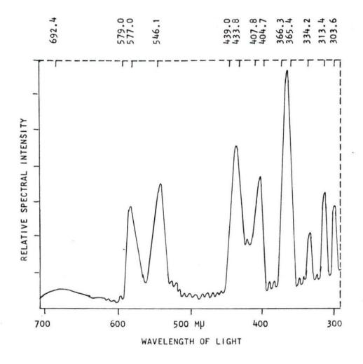
lamp housing behind a BG 38 heat filter. The transmission spectrophotogram of this primary filter is seen in Figure 5. This primary filter was used in the Leitz Ortholux research microscope adapted for fluorescence microscopy.
