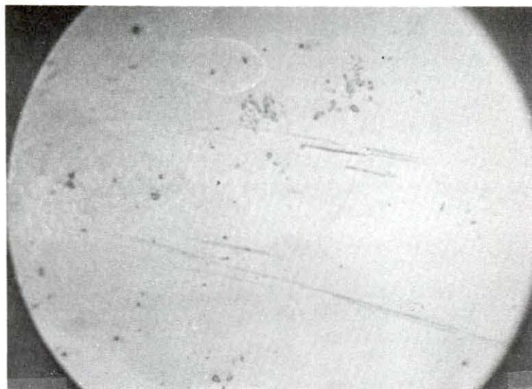
Figure 19A: post bombarded AL2 (Ti = 570°C, 99 DPA) as viewed in an interferometer without superimposed interference bands.
