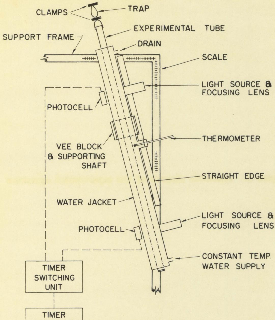
operation. The feed water was piped to the jacket from hot and cold water taps through a mixing junction. A bubble trap was installed between the mixer and the entrance to the lower end of the jacket to prevent bubbles from actuating the timing mechanism. Effluent water was piped to a drain. Fluid temperature readings were measured with a partial-immersion mercury thermometer positioned mid-way along the axis of the tube.
