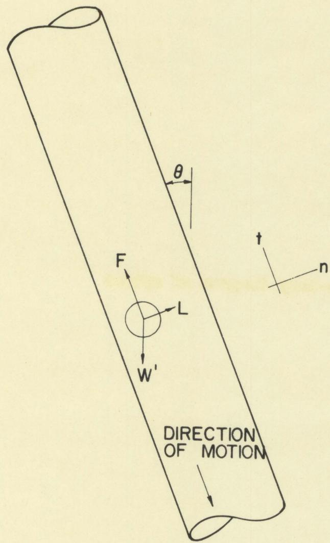
conditions are held constant, the velocity of the particle can be varied only by changing the inclination of the tube.
