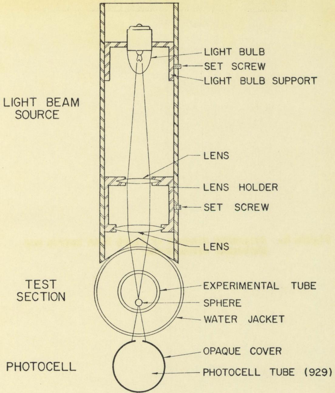
Figure 5. The experimental apparatus
