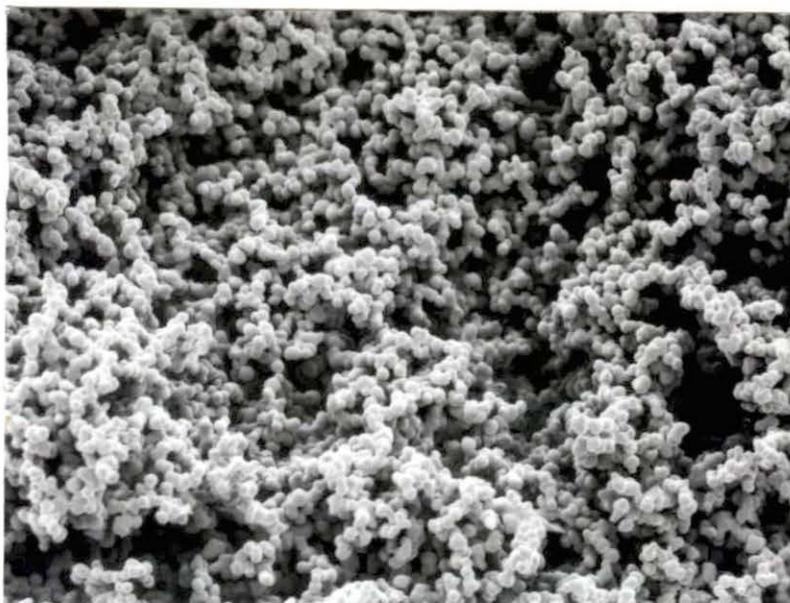
Figure 11. P-HEMA. Barvic method sample B210 with 10% initiator. 350X
