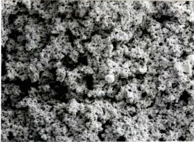
Figure 8. P-HEMA. Sample SX2 with 80% water - 20% HEMA and initiator.
