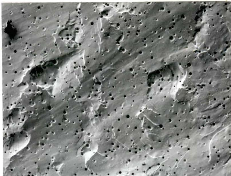
Figure 3. P-HEMA. Sample SI6 with 40% water - 60% HEMA and initiator. 350X
