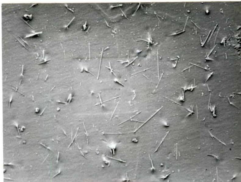
Figure 2. P-HEMA. Sample SI8 with 20% water - 80% HEMA and initiator. Small needle shaped crystals are present due to incomplete initiator removal after polymerization. 1000X
