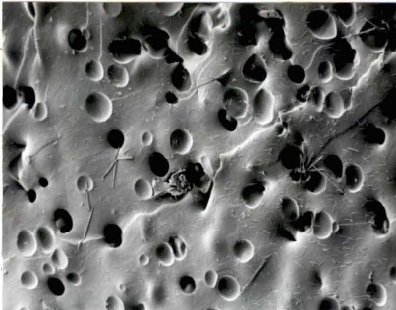
Figure 5. P-HEMA. Sample SI4 with 60% water - 40% HEMA and initiator. 350X
