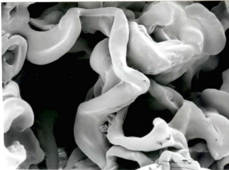
Figure 1. P-HEMA. Sample S17 with 50% water - 50% HEMA and no initiator added. 350X
