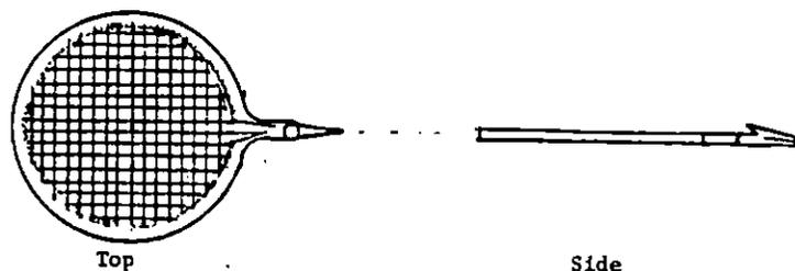
Figure 4. External defibrillation electrodes
