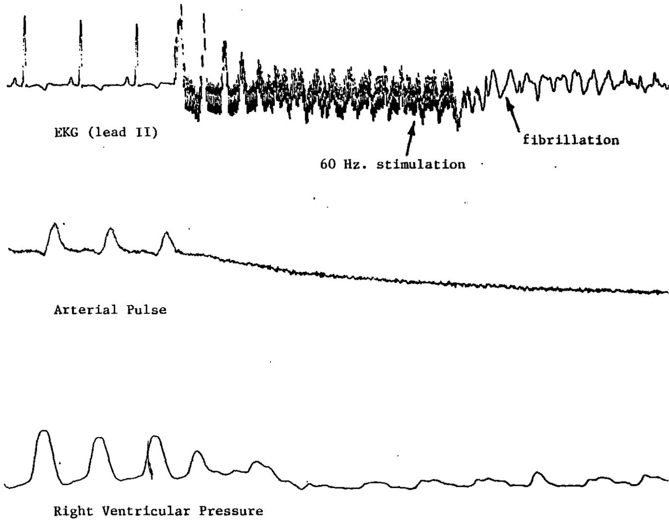
Figure 9. Fibrillation resulting from 60 Hz. stimulation
