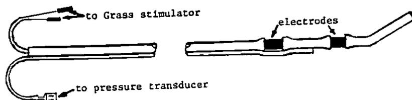
Figure 5. Stimulating catheter
