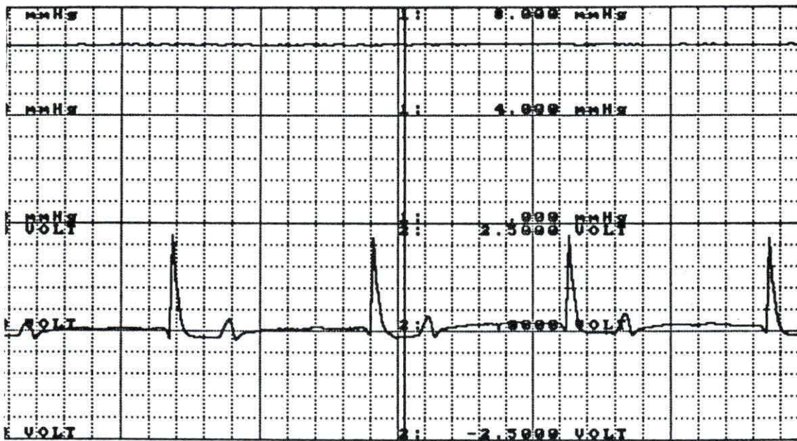
Figure A.15. A recording of venous pressure and the ECG at the start of assisting every other beat during trial #2
