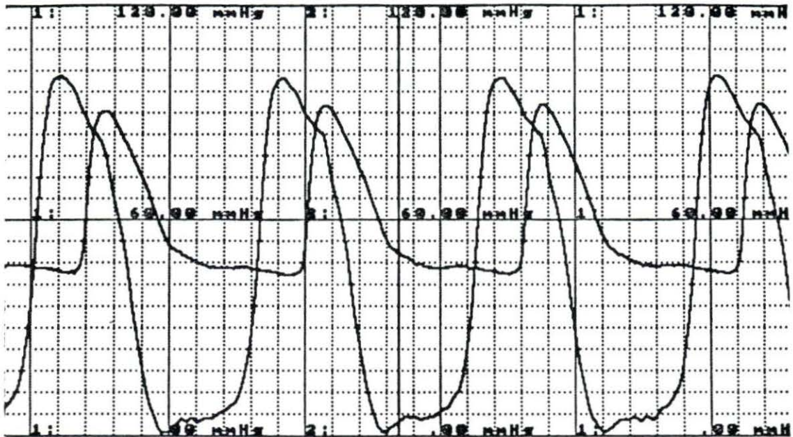
Figure A.30. A recording of aortic and ventricular pressure after assisting every beat for 15 min during trial #2
