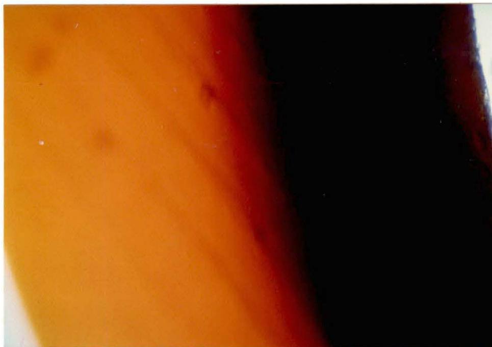
FIGURE 14. Optical microscope photograph of a cross section from the sample irradiated at 150 Krad using the formulation 60% NVP/40% MeOH and stained in Lugol/buffer (1:1) solution (magnification = 175x)
