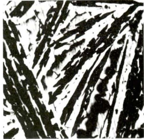
Figure 15. 71.29 a/o Pb, furnace cooled, air etched, dark area --- GdPb_2 , light area --- GdPb_3 , X50.
