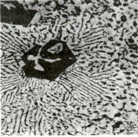
Figure 2. 15.46 a/o Pb, furnace cooled, air etched, Gd-Gd 5 Pb 3 eutectic; light area --- Gd, X200.
