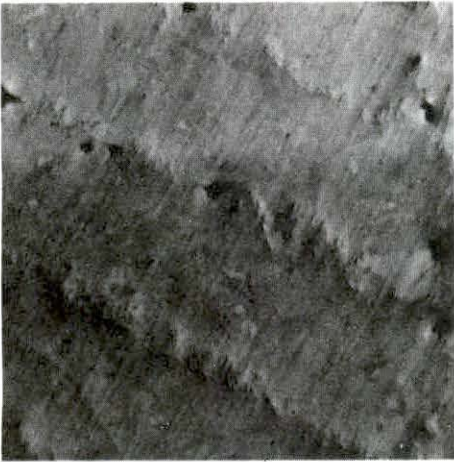
Figure 10. 47.64 a/o Pb (essentially pure Gd_{11}Pb_{10} ), furnace quenched from 1100^{\circ}C , air etched, X100.
