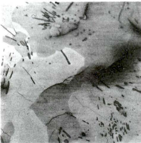
Figure 12. 53.45 a/o Pb furnace cooled, air etched, probably GdPb_2 precipitate in \sim Gd_6Pb_7 matrix, X250.
