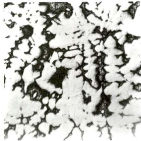
Figure 17. 78.59 a/o Pb, furnace cooled, air etched, light area --- GdPb_2 , X50.
