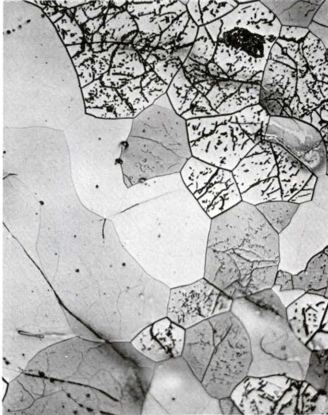
Figure 13. Metallography of PrNi<sub>5.2</sub> quenched from 1100°C (x250)
