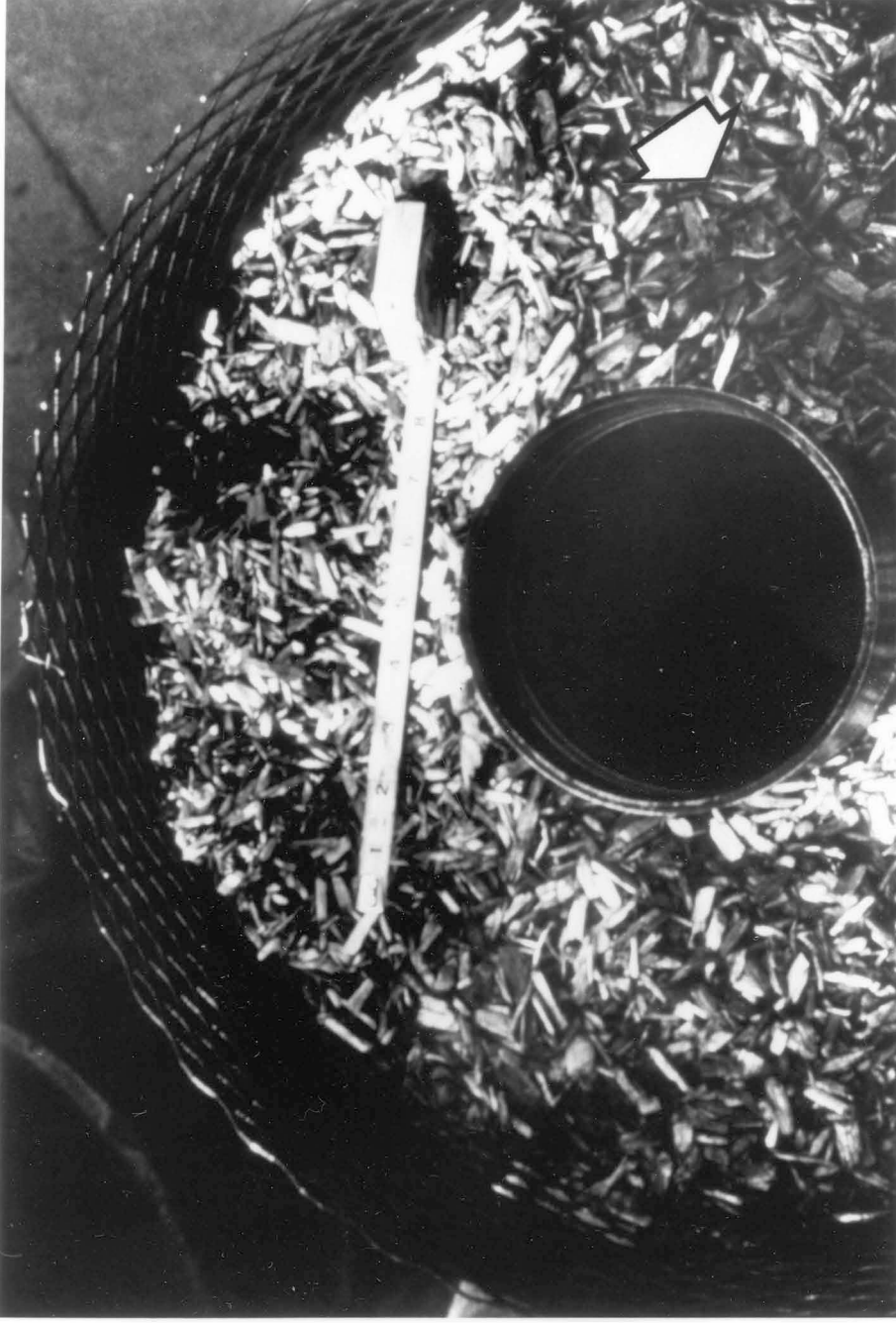
Figure 10. Wood chip filter media. The arrow identifies a pocket of pyrolyzed filter media.
