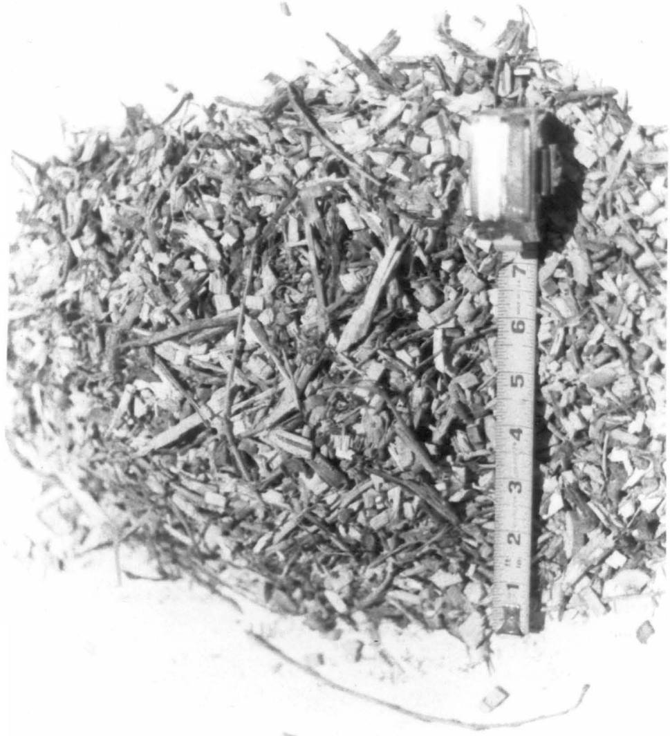
Figure 3. Sifted poplar chips harvested with a modified two row corn picker.
