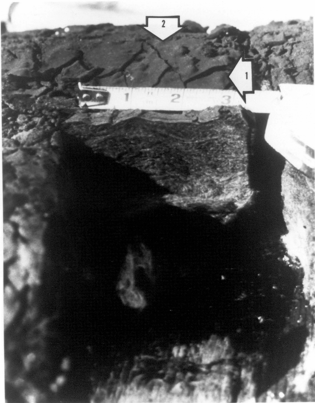
Figure 12. Outer layer of fiberglass filter media. Arrow 1 identifies the char and tar cake on the outside of the filter. Gas flow is in the direction of arrow 2.
