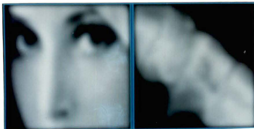
Figure 3.3: Images blurred by Gaussian shaped PSF of variance 4.0
