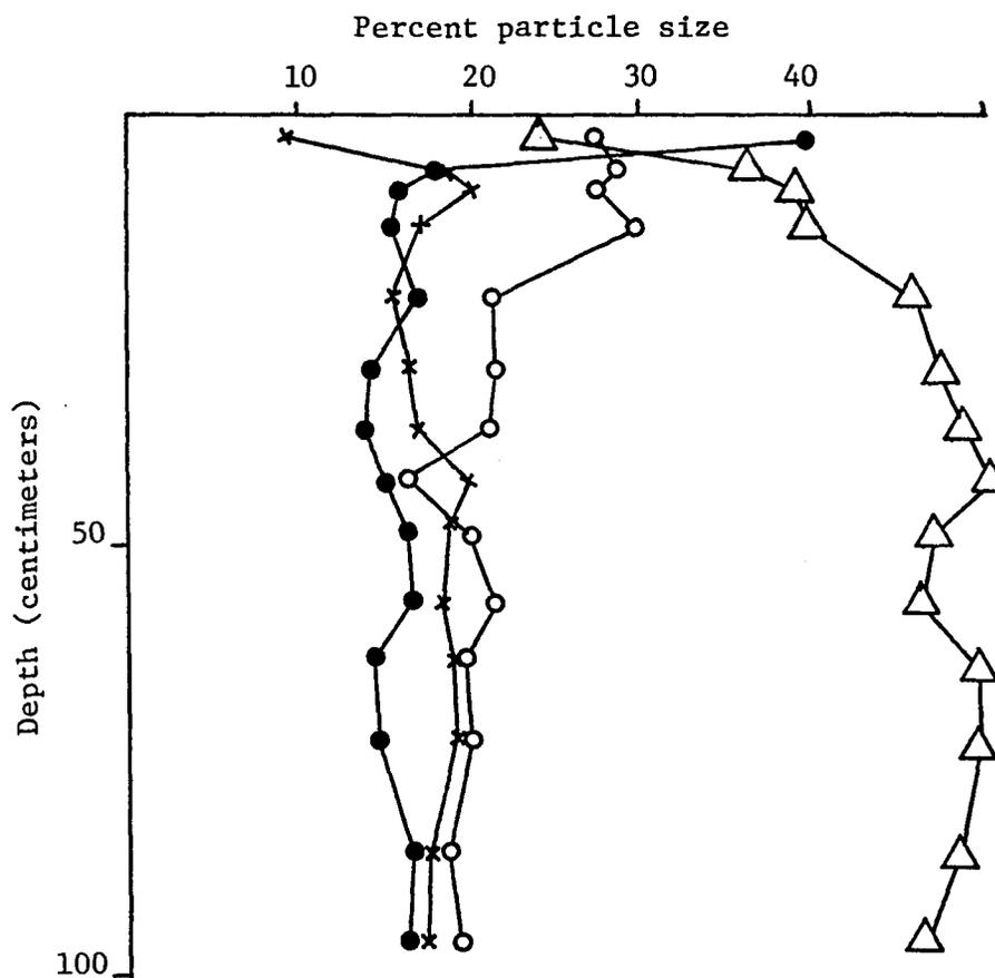
Figure 11. Particle size distribution of profile BT-3
