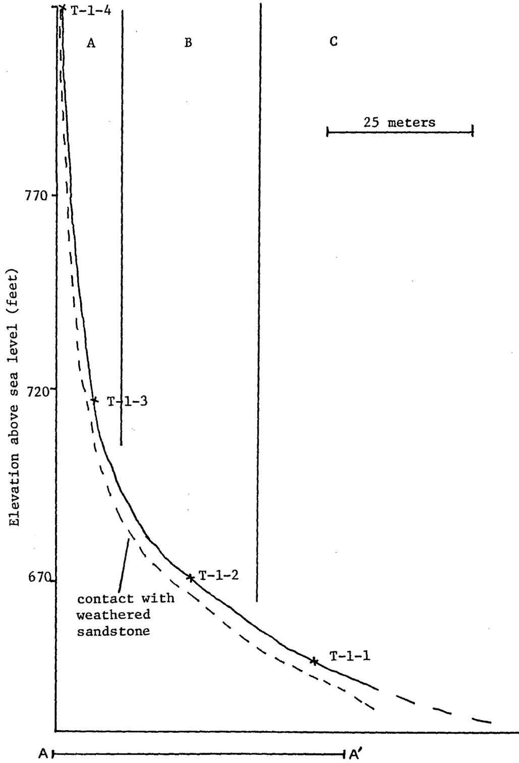
Figure 7. Schematic slope profile along Transect 1
