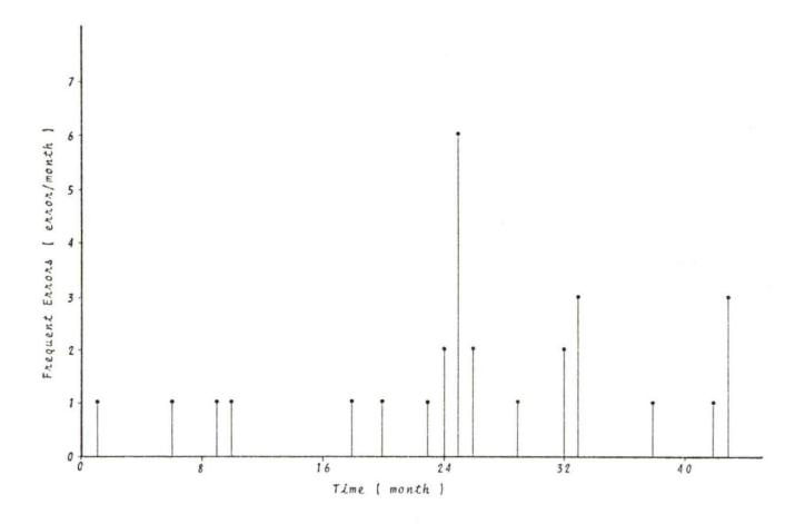
Figure 5.3. Distribution of human error for main reactor coolant system
