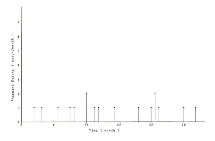
Figure 5.1. Distribution of human error for auxiliary electric power system
