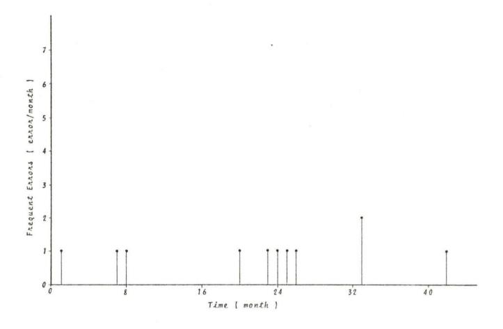
Figure 5.4. Distribution of human error for valve (component) involved
