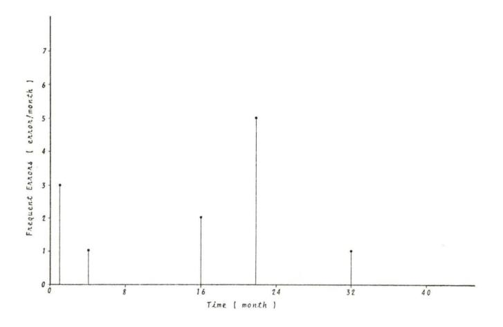
Figure 5.2. Distribution of human error for reactor protection system
